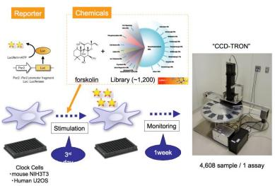
Model of the screening system used to test chemical compounds with effects on the circadian clock
